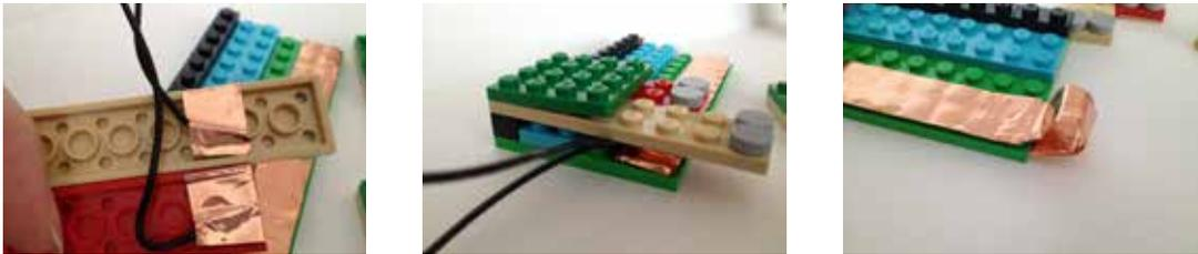
**Photos 7-9 (above)** Wires were stripped only enough to have exposed end underneath the copper tape (photo 7). Alligator clips would not fit between the pieces, so this is one option to run wiring out (photo 8) to attach clips on the other end (stripped as well) or plug directly into the back ports of the Makey Makey. The earth/ground connection had a small loop created from copper tape that allowed the alligator clip to attach securely. A wire (like the keys) could be used as instead.
