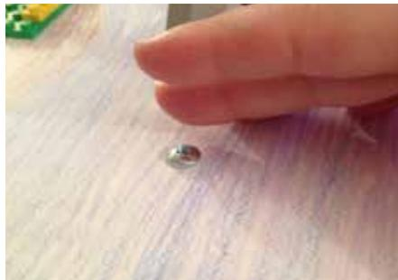
**Photo 21** The completed sample model with buttons and earth/ground connection all wired to the Makey Makey. Test the buttons by placing one hand/finger on the ground (copper tape) and use another finger to touch the top of the button (screw). This completes the circuit and triggers the corresponding sound file on the computer.
