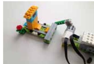
**Photos 1-3 (above)** Photo 1 shows the build for this activity “Robust Structures” that includes an earthquake simulator and 3 sample buildings (A, B and C). Each building sits on the simulator for testing. Buildings A (photo 2) and B (photo 3) can sit at the front or back of the simulator. Building C sits in the middle (photo 4).
