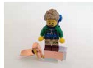
**Photos 4-6 (above)** Variations on using the switch with a "cap" on top (photo 4) or an open top (photo 5) that allows a mini figure to be attached (photo 6). Again, the copper tape would need to be adjusted/trimmed to accommodate an area for where the model is touched when adjusting the switch.
