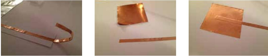
**Photos 4-6 (above)** Photo 4 shows the ground connection tab created from the thin strip of copper tape. The tape was folded back on itself to create the tab that sticks out. The top of the switch has the same thin copper tape running to the edge (photo 5) but also has a larger square of copper tape smoothed on top (photo 6) to provide a greater surface area to trigger the switch.
