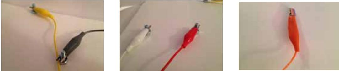
**Photos 16-18 (above)** Use alligator clips to attach each button to the Makey Makey. Note that each button should connect to the appropriate port on the Makey Makey to correspond with the Soundplant keymap (or Scratch program). Encourage students to test these before taping (if needed).
