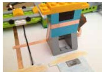
**Photos 19 and 20 (above)** Photo 19 shows that the building can be placed on the simulator the same way. The copper tape does not interfere in this case since the model does not need to stick to studs (it sits on the simulator, not connected). Photo 20 shows the third option illustrated with building C completed and in place to make the connection. Touching the tab on the right side, while the model is in place touching the ground strip, will complete the circuit and trigger the Makey Makey.
